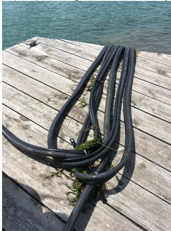
Pre-deployment (above); post deployment (below) reveals tangle around brackets that may have interfered with performance.
